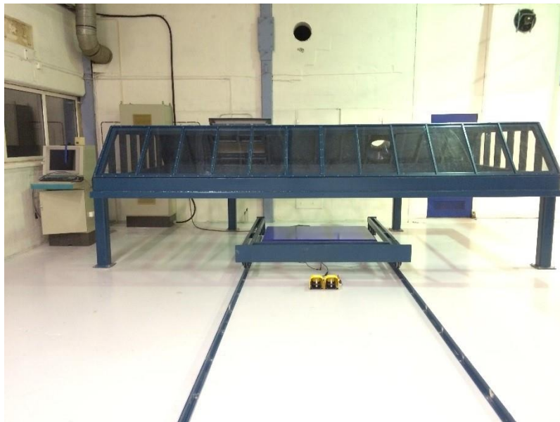
Wind load tester 4,90 m x 2,65 m
