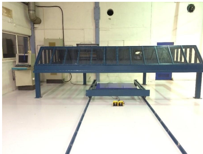
Wind load tester 4,90 m x 2,65 m
