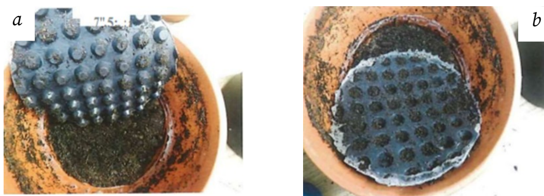
Fig. 9. Testing of profiled membranes for resistance to root – proof: a , b – the sample of the profiled membrane did not allow the roots to germinate
