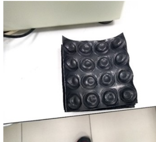
Fig. 4. Example of testing a sample of a profiled membrane with a size of 10x10 cm for compression
